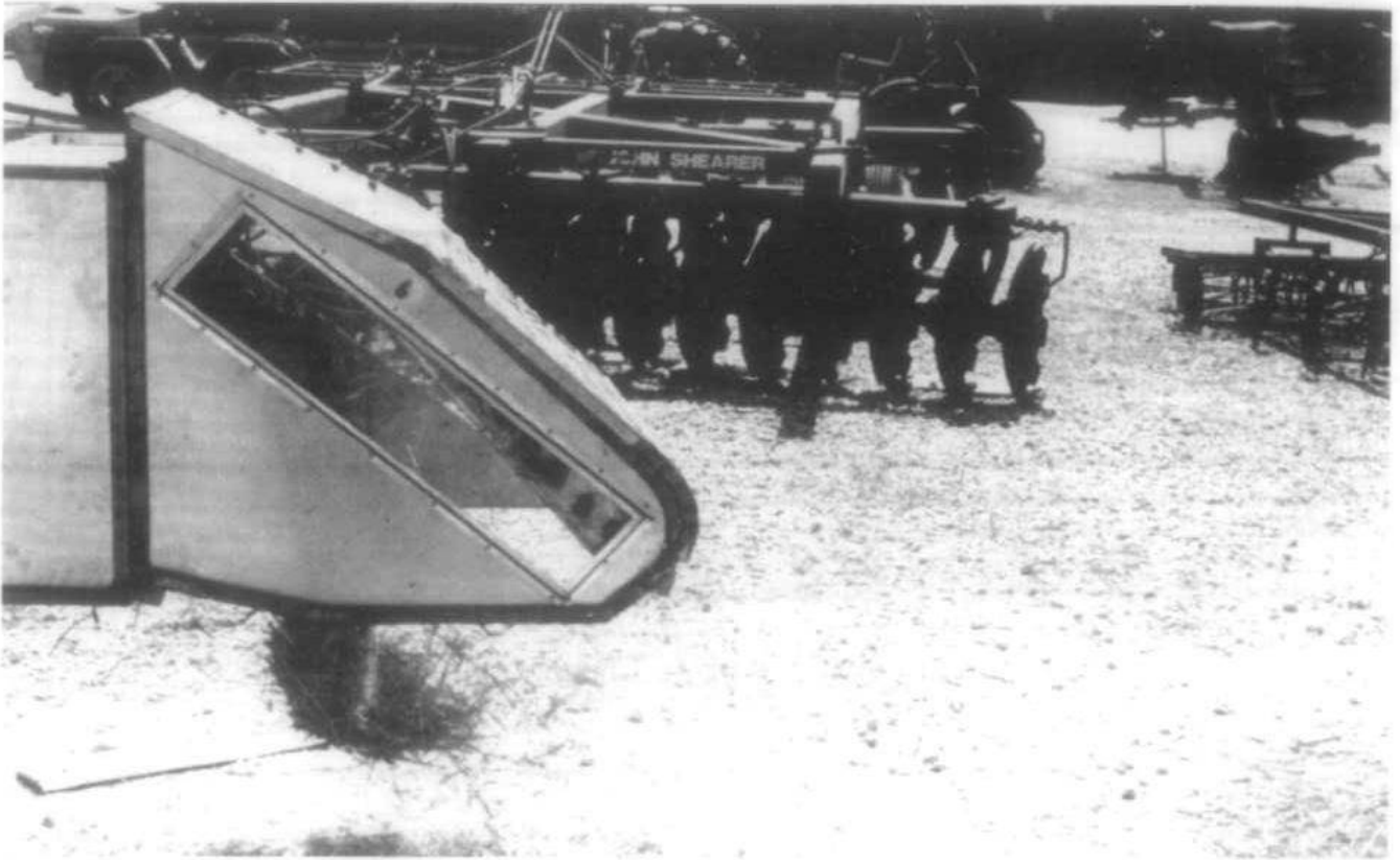
Fig. 12: The collector without the collecting bag showing the diverted bulk straw
