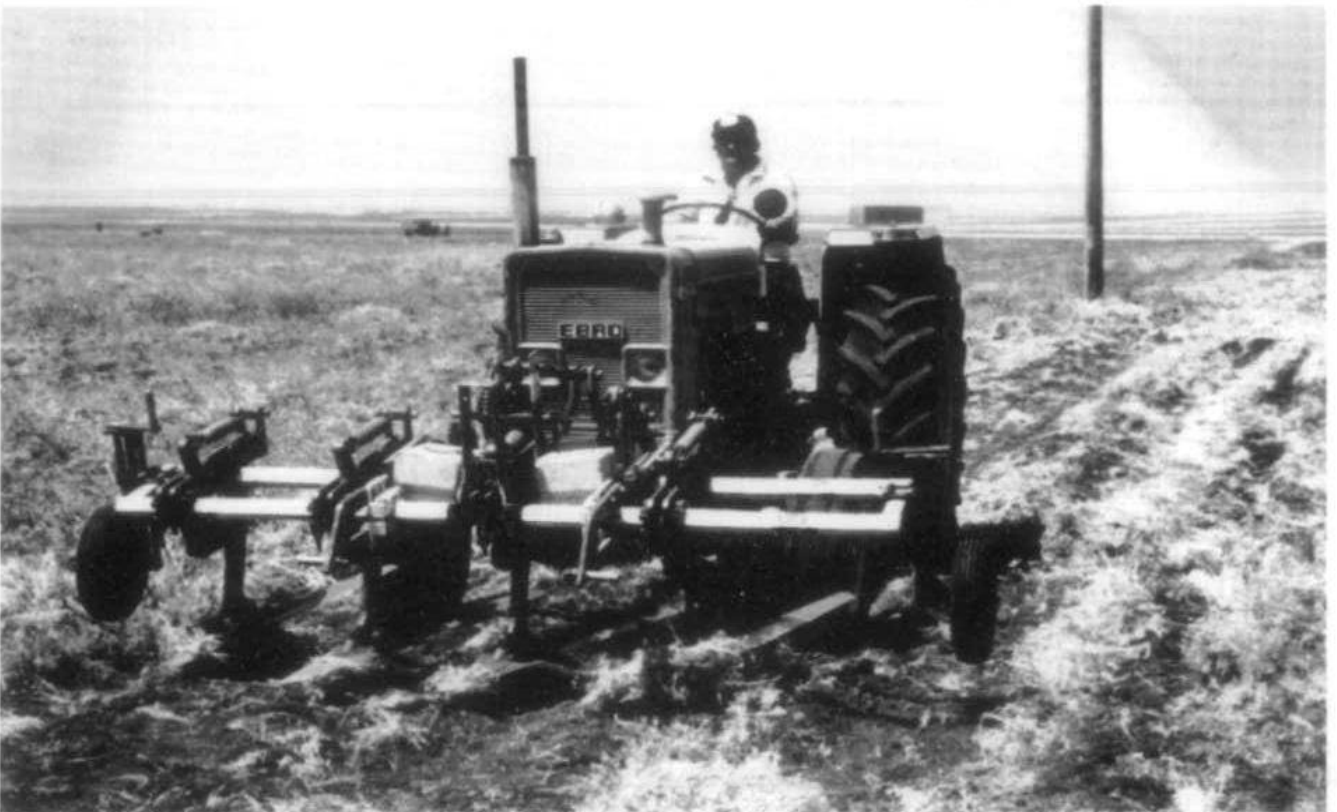
Fig. 5: Front-Mounted Angled-Blade Cutter with locally manufactured EBRO-tractor during Lentil Harvesting (IDRC-Project)
