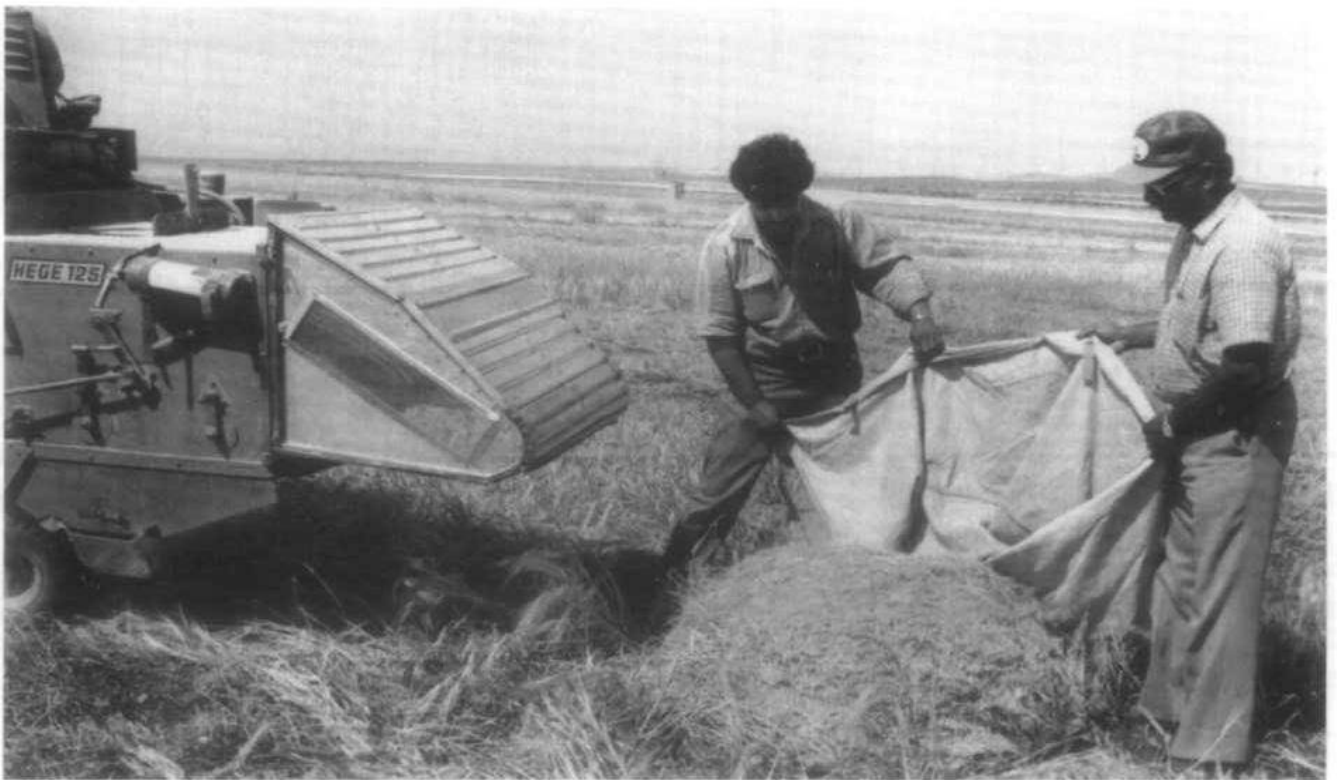
Fig. 13: Removing the straw and chaff from the collecting bag
