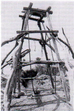
Figure 1: Traditional wooden drilling rack as being used until the 80ies in the Egyptian Dakhla Oasis.
